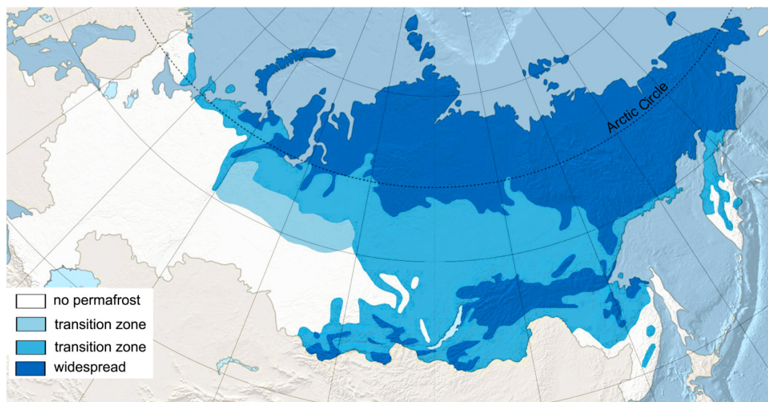
Fig. 1. Permafrost distribution in the Russian Federation (Kotlyakov and Khromova 2012). Zones represent the permafrost density and thickness. Permafrost depth in region 2 is above 50 m, in region 3 it is 50–90 m, and in region 4 it is below 90 m. [Colour online]
